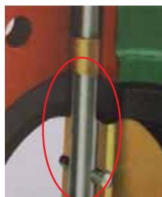
No second sealing. Stem connected by pin, which may cause leakage and by vibrations or high torque, it can shake out or break.
