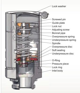
Spring-loaded vacuum relief valves are used as vacuum limiting valves in pipelines or pressure vessels. If the vacuum in the pipeline or pressure vessel reaches the force set by a spring, the valve opens and air can flow into the pipeline or pressure vessel through the intake slit in the valve body. The valve closes once the set vacuum pressure is reached again.
