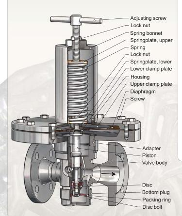
Pressure reducing valves are independent of the primary pressure and, depending on the pressure range, are either piston or membrane controlled, spring-loaded proportional regulators. They are used to maintain the reduced pressure at a constant, adjustable set value.
