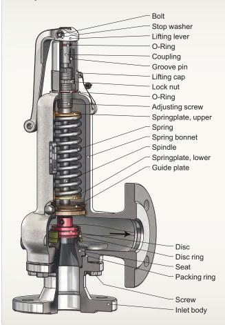
Spring-loaded safety valves can be used as fittings with a safety function in pipelines and on pressure vessels.
