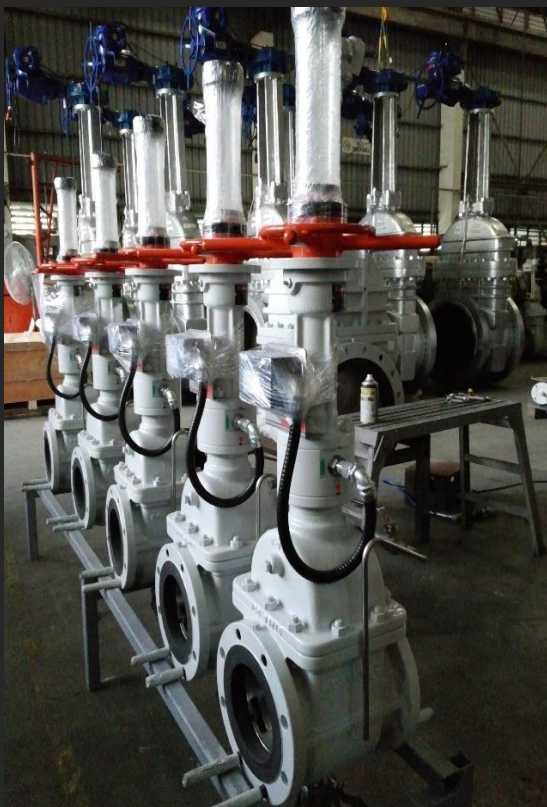
DBB Valve with Proximity Sensors
