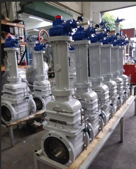
Rising Stem Valves with TGM Gear Operators
