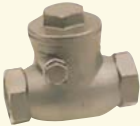
SW-200 Swing Check Valve • Size: 3/8" - 3" • 200 PSI • Body: CF8M
