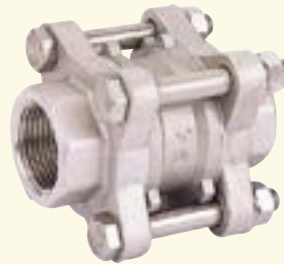
SLC-3 3-Piece Spring Loaded Check Valve Size: 1/4" - 4" 1000 PSI max. Body: CF8M Ends: Threaded, Socket Weld, Butt Weld
