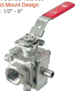
SERIES 88J Direct Mount Design Size: Full Port 1/4" - 1 1/2" Reduced Port 1/2" - 2" 2000 PSI max. Ends: TH, SW, BW, FL
